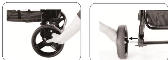
Press the wheel release button in the middle and pull out the wheel to remove it from the axle.
