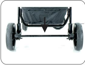
**TO BRAKE THE STROLLER:** Press down firmly on the brake pedal's / linkbar by foot.
