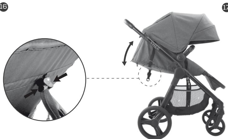
Squeeze the backrest reclining adjuster to adjust the position of the backrest.
