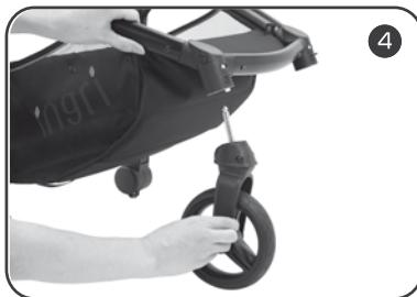
Fix the front wheel axles into front legs houses, it is fixed when you hear a CLICK.
